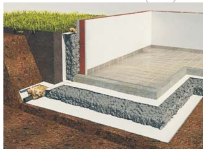
Perimeter insulation flanking the floor slab and basement wall
