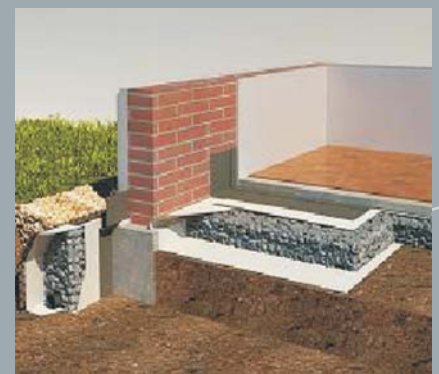
Floor insulation older building/restoration
