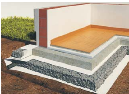
Perimeter insulation under the floor slab
